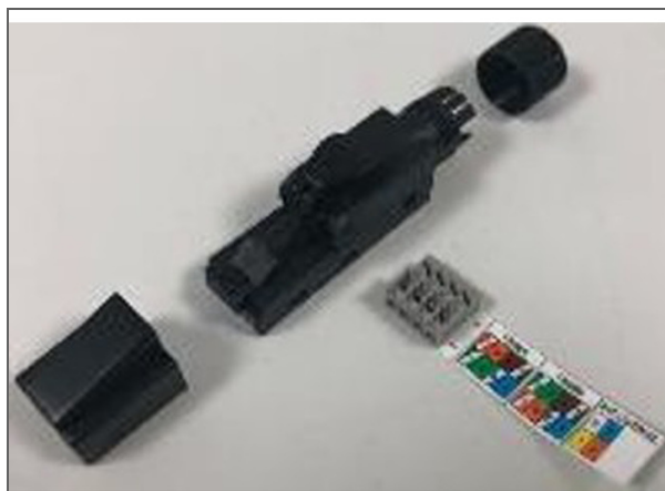
RJ45 field-installable connector Category 6A UTP Straight
